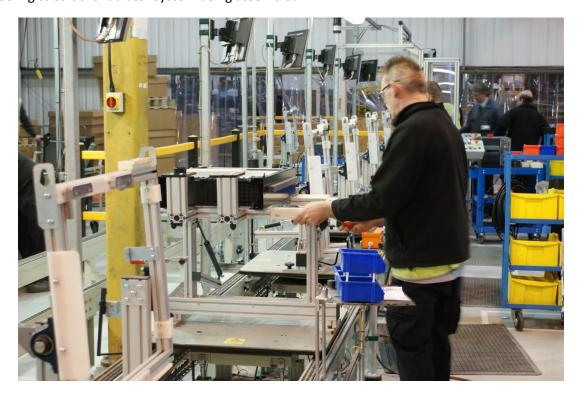
There are 4 manual workstations, a leak test station and an unload station along the front edge of the conveyor, the opposite side of the conveyor is simply used to return empty pallets back to the start. of the process.
