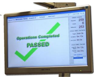
This custom designed and manufactured system provided a cost-effective solution to ensure the correct assembly process was adhered to by the operators and combined a final leak test as a quality assurance check for the final automotive radiator assembly. This type of special purpose machine is ideal for low volume production of many different variants of parts. New design of parts can be accommodated along the same assembly line by simply designing and manufacturing new tooling pallets.
