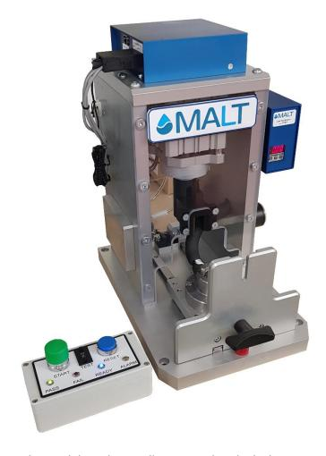
An OEM MALT LT201 valve module and controller are used as the leak testing instrument, with the valve module mounted close to the fixture tooling to keep the test volume as small as possible. A button box is included for operator controls, this was on a flying lead to be positioned either to the right or left of the drawer for right or lefthanded operators.
