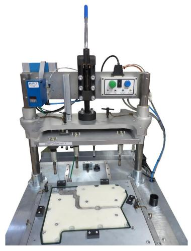
An OEM MALT LT401 valve module and controller, complete with a button box is mounted onto a standard series 10 flexible leak testing system and allows leak testing of medium-to-large aluminium die cast parts.
