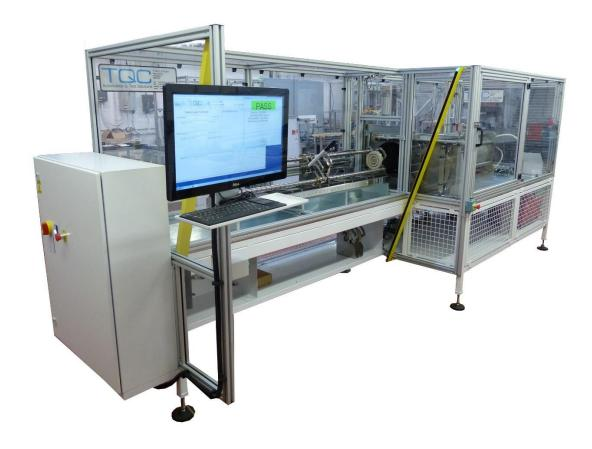
This system allows the operator to load the tooling with a fuel pipe, securing 2 off end clamp units, followed by automated testing. The fixture is advanced into the test chamber, a door then closes and seals the test chamber. The automated test begins with a high pressure proof test and if successful moves onto the helium leak test. On completion of the testing the chamber and part vent to ambient followed by opening of the chamber door and transfer of the test piece ready for manual unloading.
