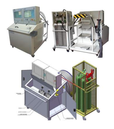
The system also has a bar code scanner to identify both the wing and the test operator. The system interfaces to the clients Management Information System for archiving test results, downloading test protocols written offline and for authorisation of test personnel.
