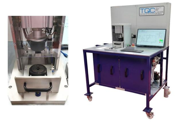
This system allows the operator to load the tooling nest located in the drawer, the drawer is pushed forwards to the closed position to allow automatic leak testing.
